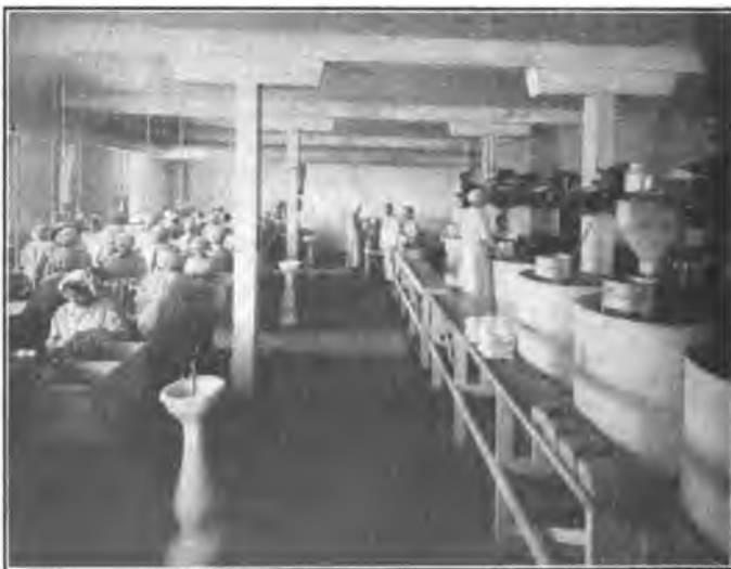
FIG. 69.—Breaking eggs (on the left). Mechanical mixer to prepare eggs for freezing (on the right). (By permission Seymour Packing Co.)
